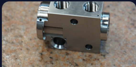
Surface finish closeup — face-milled stainless steel achieving Ra 12.4 \mu\text{in} (0.31 \mu\text{m} ).
