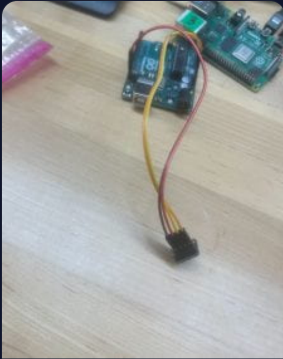
Assembled PPG circuit — MAX30102 sensor breakout soldered with header pins, connected to Arduino Uno via I2C (SDA/SCL), powered via USB.
